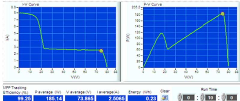
② There's shadow at the top left corner of PV module, the tracing efficiency is 99.61%.
