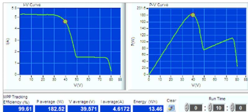
③ Simulate tree shade covered PV module, the tracing efficiency is 97.49%.
