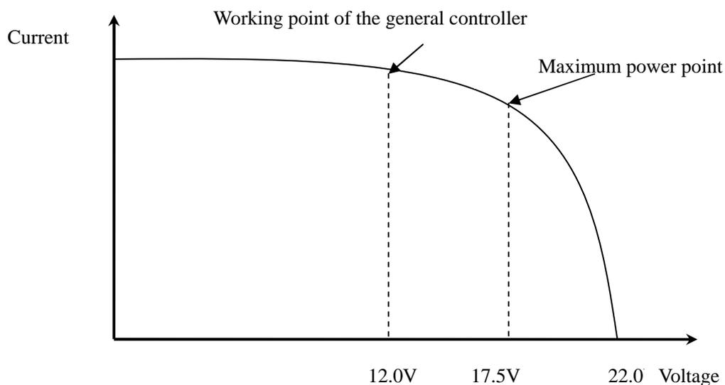
As a charging stage, MPPT can't be used alone. It must be combined with ascending charge, floating charge, equalizing charge to complete the battery charge.
