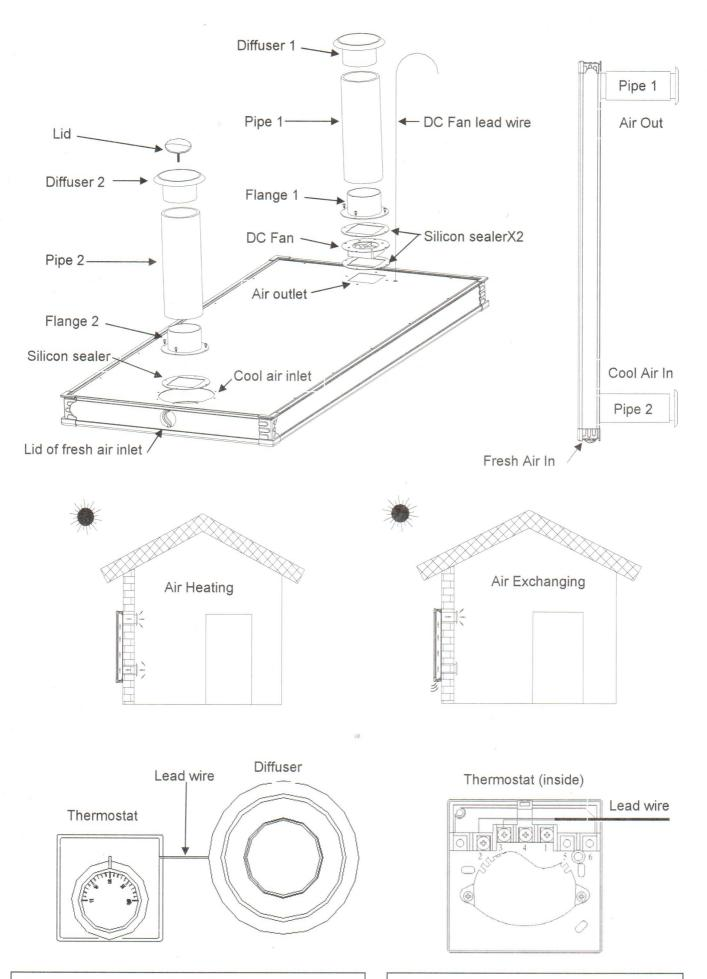
Secure thermostat onto the inside wall near the diffuser Connect lead wire from solar heater to thermostat
